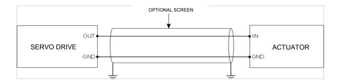
To prevent signal corruption, a shielded cable should be used.
