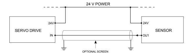
Since 4 to 20 mA signals are inherently resistant to electrical interference, the wiring can be made using common unshielded cable in many cases. However, shielded cable is preferred when the wiring extends over great distances or through particularly unfavourable environments.
