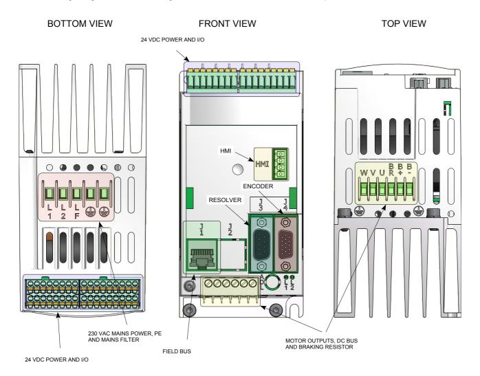
The Miniaction 300 is also equipped with a stage for piloting the braking resistor.
