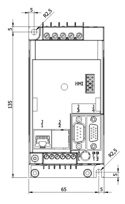
Since the servo drive heats up during operation, at least 100 mm of obstacle-free space must be left at the top and bottom to allow air to flow uniformly around the device.
