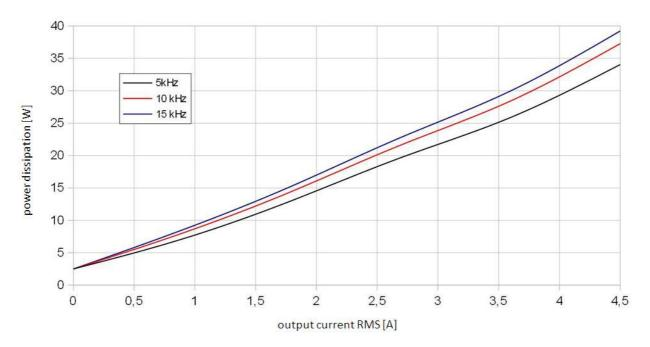
Since the current that can be delivered by the servo drive depends on ambient temperature, a cooling system must be provided in order to prevent a reduction in actual deliverable current, when necessary.
