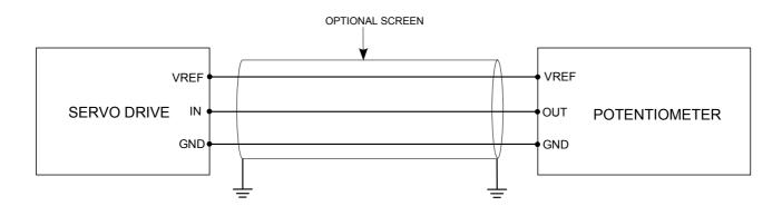
In both cases, shielded cable should be used for connection.
