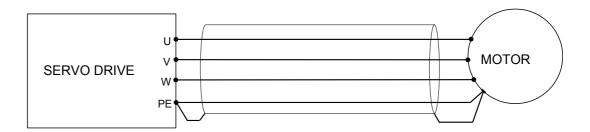
The motor is connected as shown in the following figure:
