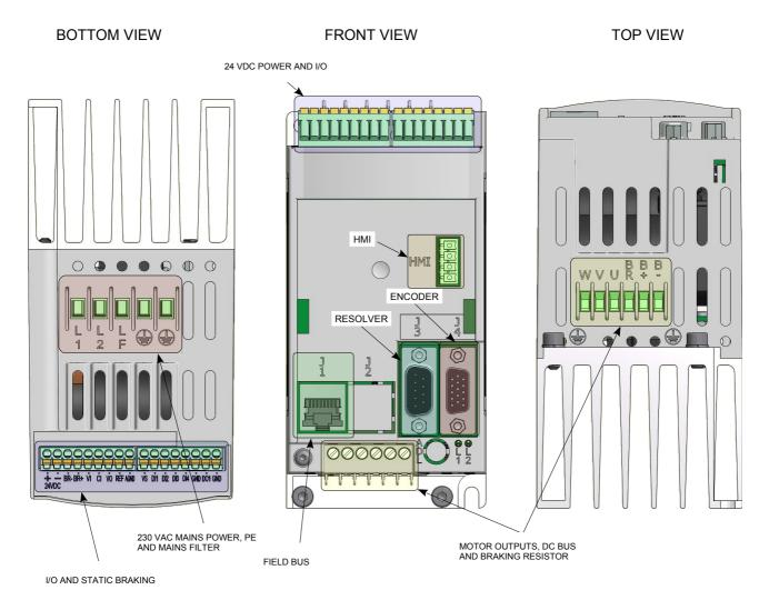
The Miniaction 200 is also equipped with a stage for piloting the braking resistor.
