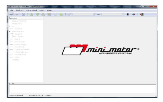
To proceed with the update, the communication port in the MiniMe software must be programmed.
