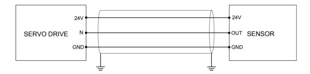
Since the input stage has a relatively wide passband to allow acquisition of high frequency signals, it is particularly susceptible to electrical interference. Therefore, be sure to use shielded cable to make the connections. In this case, the shield must be connected to earth on both sides, preferably with a low-impedance connection such as a metal cam. The shield is completely ineffective if it is left floating.
