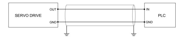
In this case, since there is greater likelihood of electrical interference problems, use shielded cable to make the connections. The shield must be connected to earth on both sides, preferably with a low-impedance connection such as a metal cam. The shield is completely ineffective if it is left floating.
