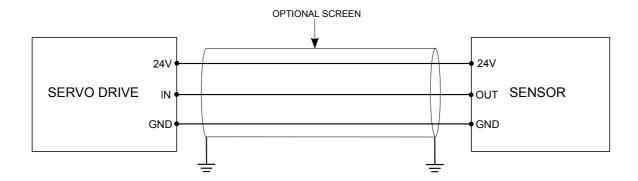
However, if the operating environment is affected by significant electrical noise, or if the distances to be crossed are significant, the use of shielded cable may be necessary. In this case, the shield must be connected to earth on both sides, preferably with a low-impedance connection such as a metal cam. The shield is completely ineffective if it is left floating.
